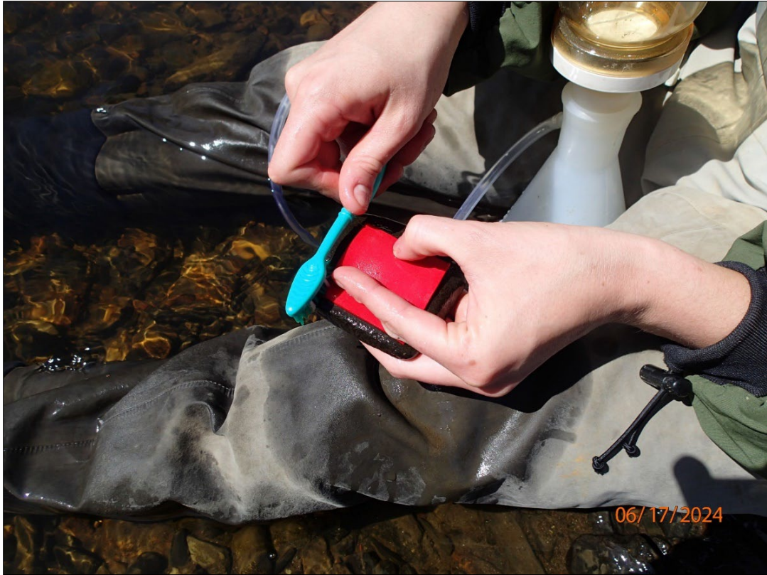
Figure 3.—Brushing/removal of material from rock around the flexible foam square.
