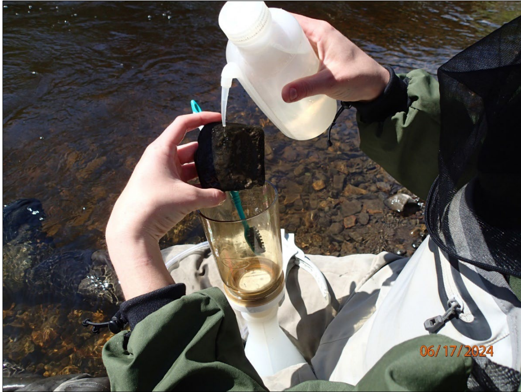
Figure 5.—Removal of material remaining beneath the flexible foam square and rinsing with clean water into the filter receptacle. Note toothbrush is placed in the filter receptacle since it contains part of the sample material.
