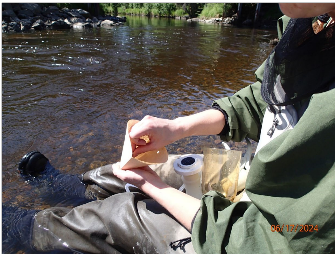
Figure 6.—The folded glass fiber filter is placed in a coffee filter. The coffee filter is folded to completely cover the sample glass fiber filter.
